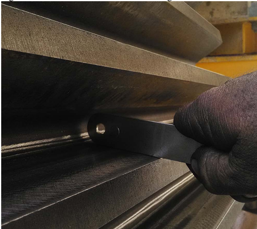
Fig 9: View of profile after finishing – some of the wear step has been taken down.
