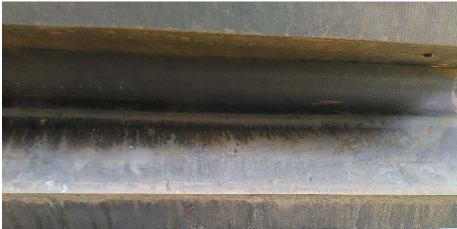
Fig 3 Non drive end of girth gear before remedial work.
