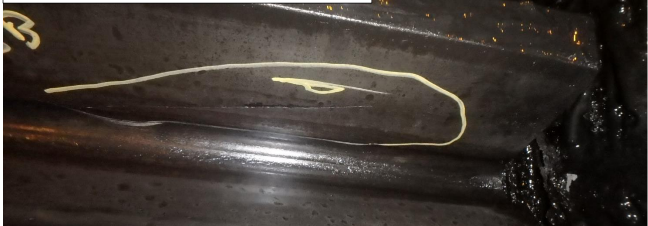
Fig 1 Crack on unloaded side of tooth 393 March 2019
