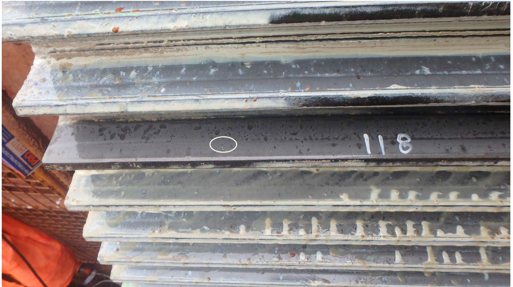
Tooth 118 highlighting the isolated pit.
