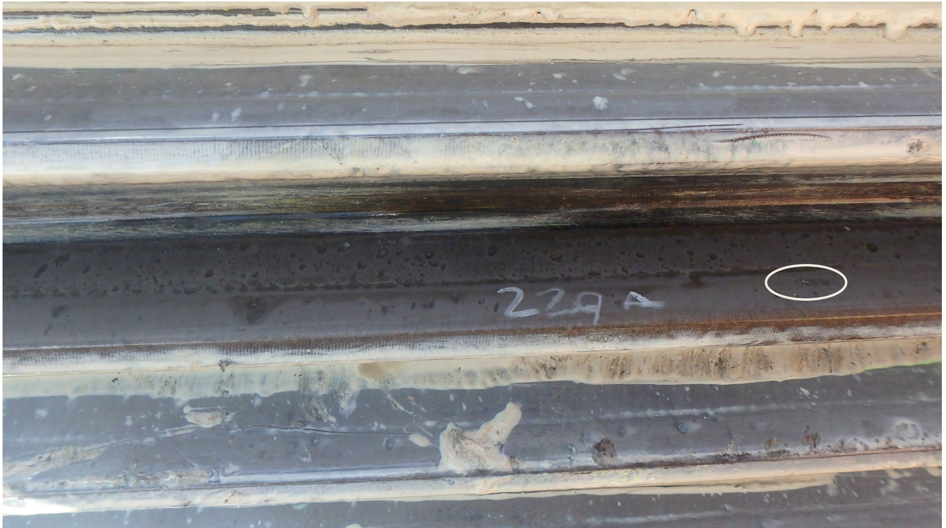
Tooth 229 showing a localised pit.
