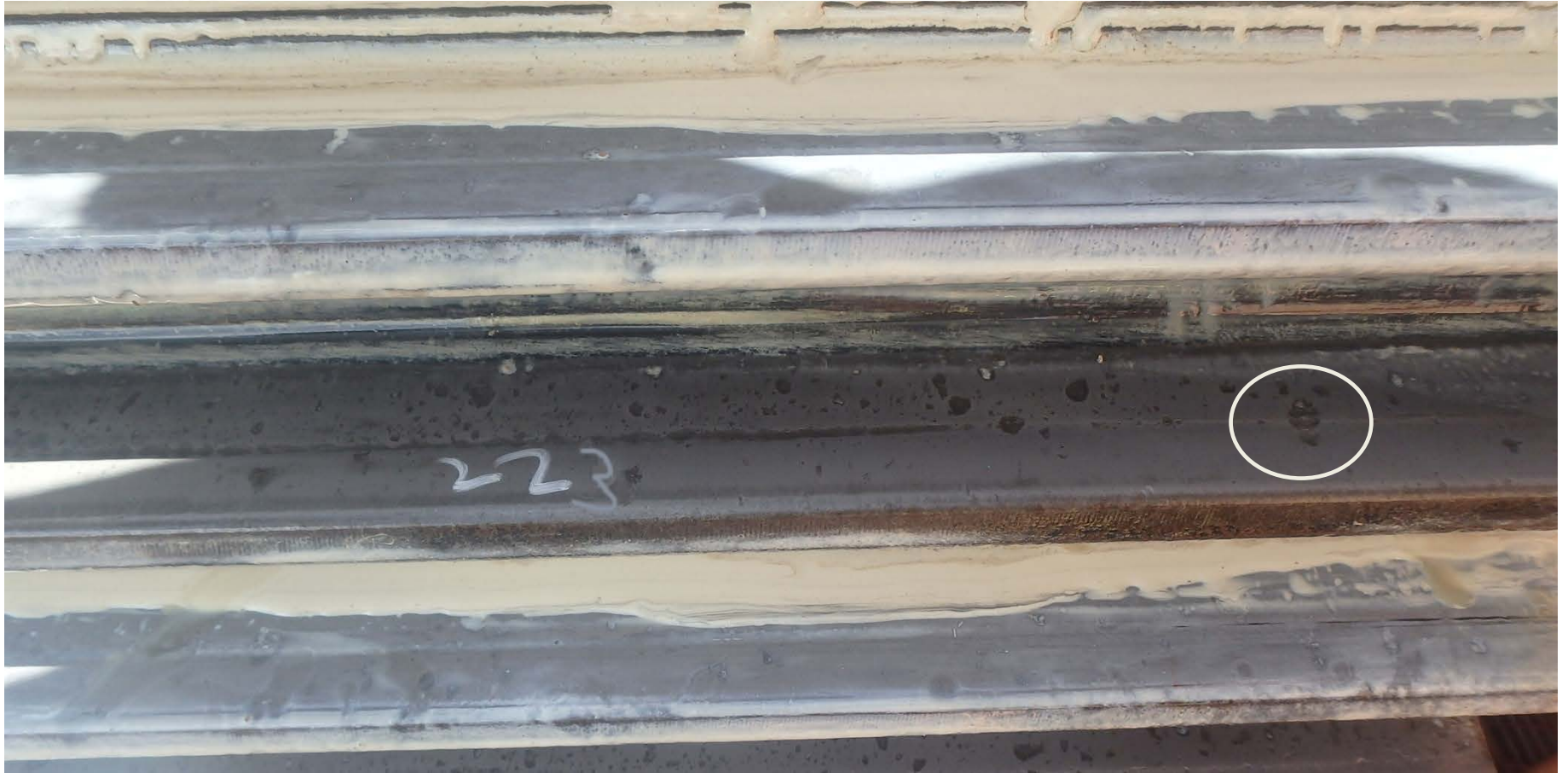
Tooth 223 A - minor surface breaking anomaly apparent
