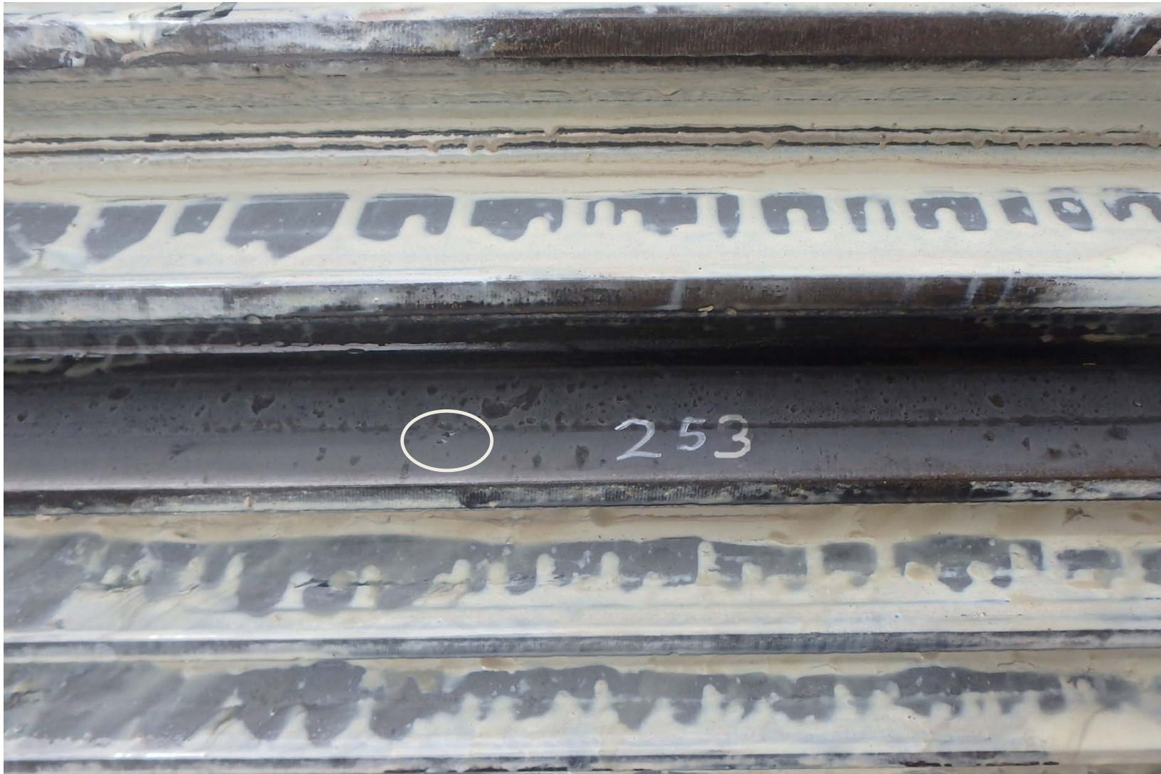
Tooth 253A highlighting the isolated anomaly.
