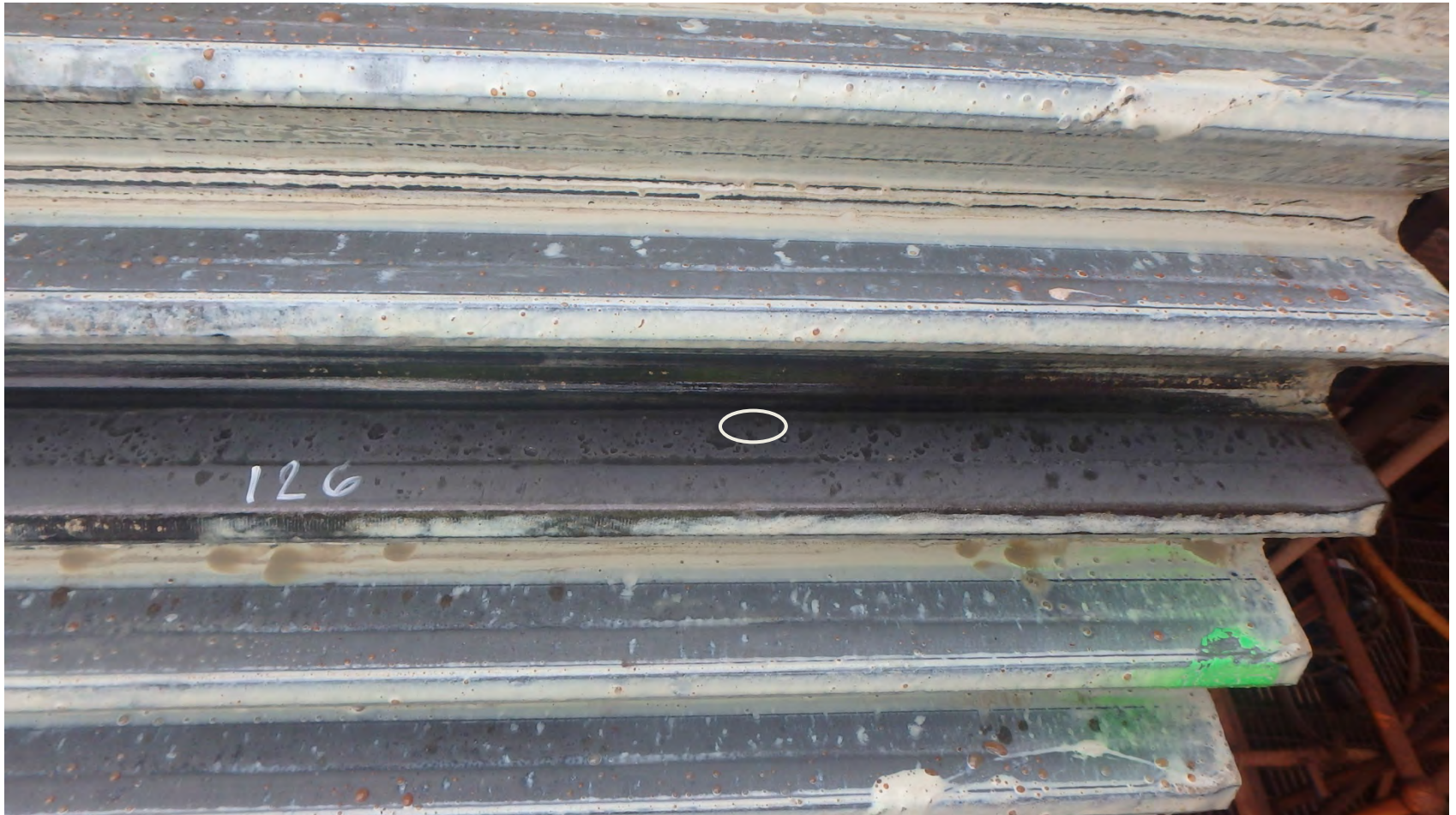
Localised anomaly in the root of tooth 126 A.
