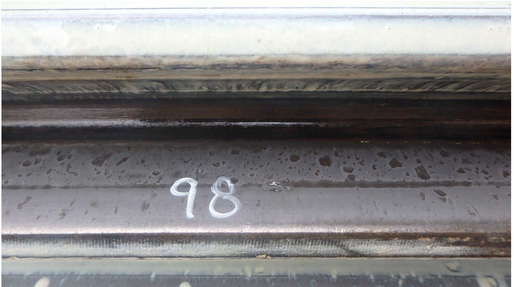
Fatigue pit found on tooth A 98.
